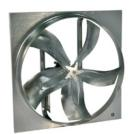
Designed for commercial and industrial applications requiring high volumes of air at low static pressures. Construction includes heavy-duty drive frame rails and one-piece motor/bearing plate. Propeller utilizes a five-blade reinforced galvanized steel design which provides low sound levels. Mount in vertical position for exhaust applications or horizontal position for supply applications.
