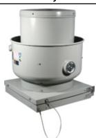
Designed for heavy grease applications as found in char broilers, solid fuel cooking, and Oriental cooking. Fans are UL 762 listed for all electrical components and grease removal. Units are constructed of heavy gauge steel and utilize a one-piece steel windband that is continuously welded to the curb cap. Clean out port, heat baffle, Nema-
