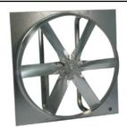
Designed for commercial and industrial applications requiring high volumes of air at low static pressures. Construction includes rigid drive frame rails and one-piece motor/bearing plate. Mount fan in vertical position for exhaust applications or horizontal position for supply applications.
