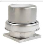
Designed to meet the general clean air exhaust requirements for industrial and commercial buildings. Features a fully rolled windband bead for increased stability and easy transport. Fresh outside air is drawn in under the motor cover to maximize motor life.
