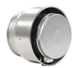
Designed for use in restaurants, schools, commercial, and industrial applications to exhaust contaminated air from kitchen range hoods, up and away from the roof. Leakproof, spun aluminum construction features a fully rolled windband for increased stability.
