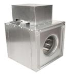
Designed for indoor clean air applications including intake, exhaust, return, or make-up air systems in industrial or commercial buildings. Rugged construction allows fan to be installed in ductwork either horizontally or vertically. Duct collars provide easy duct connections. Access panels are included on each side of the unit. • Aluminum backward inclined, nonoverloading centrifugal wheel design
