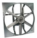
Designed for commercial and industrial applications requiring high volume of air at low to medium static pressures. Construction includes heavy-duty drive frame channels, bearing plate and motor plate. Propeller utilizes a six-blade heavy-duty cast aluminum design. Mount in vertical position for exhaust applications or horizontal position for supply applications.
